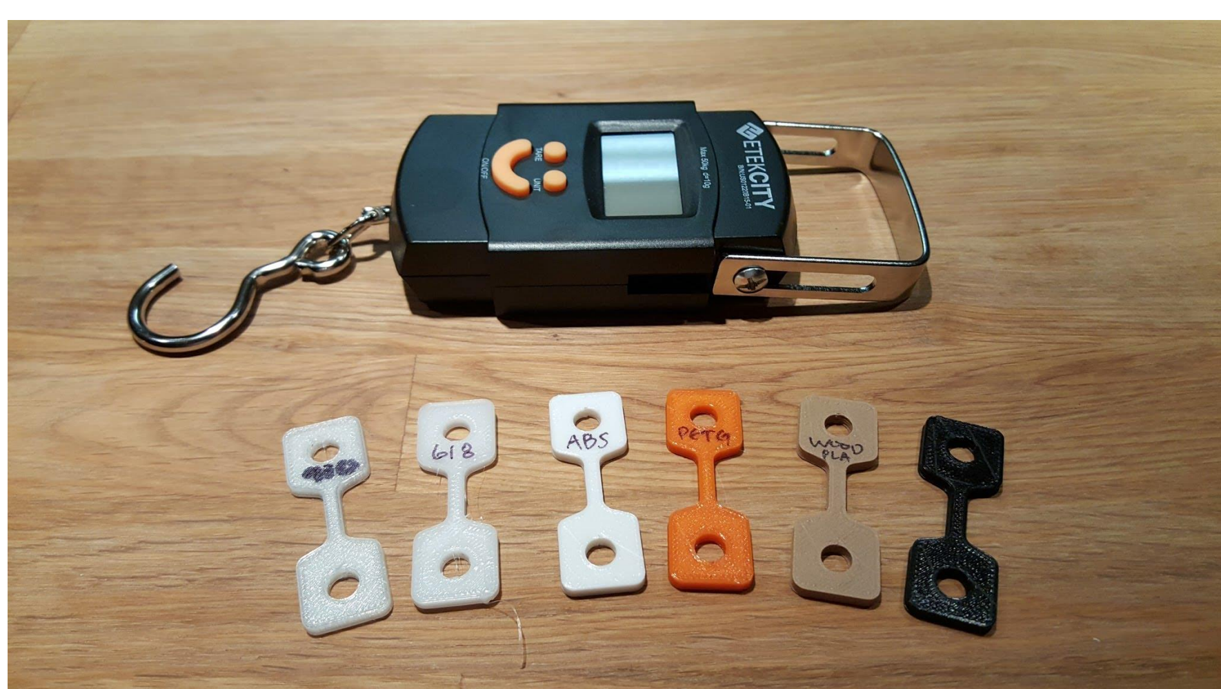
Fig 3: A force meter is used to determine how much force is needed to completely break the test object of various materials. ABS, PLA, PETG, and TPU were the subjects tests
