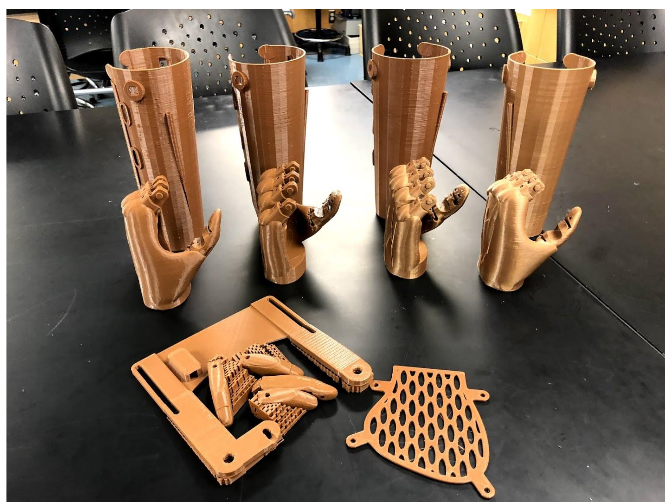
Fig. 1: Finished printed Gripper hand models by using the design in collaboration with Grit3D. The hand functions by provided the basic needs of a hand. The mechanism provides a gripping mechanism to be able to grasp round and flat objects.
