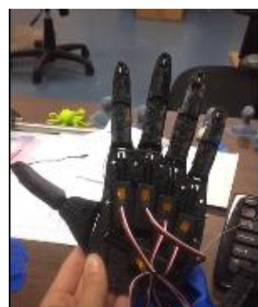
Fig. 4: This is the final prototype design that has been developed. This is paired with a commercially available Myoelectric Armband from Thalmic Lab ( https://www.myo.com/ ). This system allows for 5 different poses. The hand, which houses 5 linear actuators to control individual finger motion, is the open source Ada hand design from Open Bionics ( https://openbionicslabs.com/downloads/ ). The arm is designed using solid body modeling in Fusion 360 and mesh-refinement in Meshmixer based on a 3D scan of PI Gagnon's arm. The project took 6 weeks to complete and has been adjusted to be easier for the general public to be able to afford and replicate. In total this prototype would be about $350 dollar, $130 due to the 5 linear actuators, $200 for the Myo gesture band, the rest is for batteries, wiring, and the plastic for the casing of the prosthetic.
