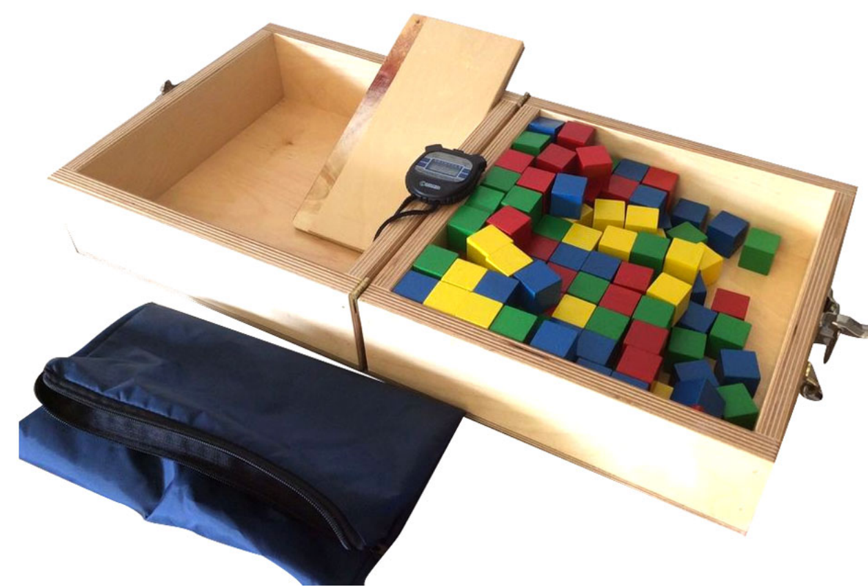
Figure 1. The simple components of a box and block test. This dexterity test is easily replicated worldwide and can serve as a benchmark for current and future hand designs.
